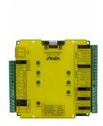
The KDH-KS3012-IP standard controller is designed to work with the new NMS AC physical access control system. Communication with the system server is based on TCP/IP protocol via the Ethernet port on the controller board.
