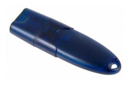
A license in the form of a hardware USB key enabling connection of 8 devices following the RTSP/HTTP protocol to NMS NVR recorders and MMS software installed on a PC.
